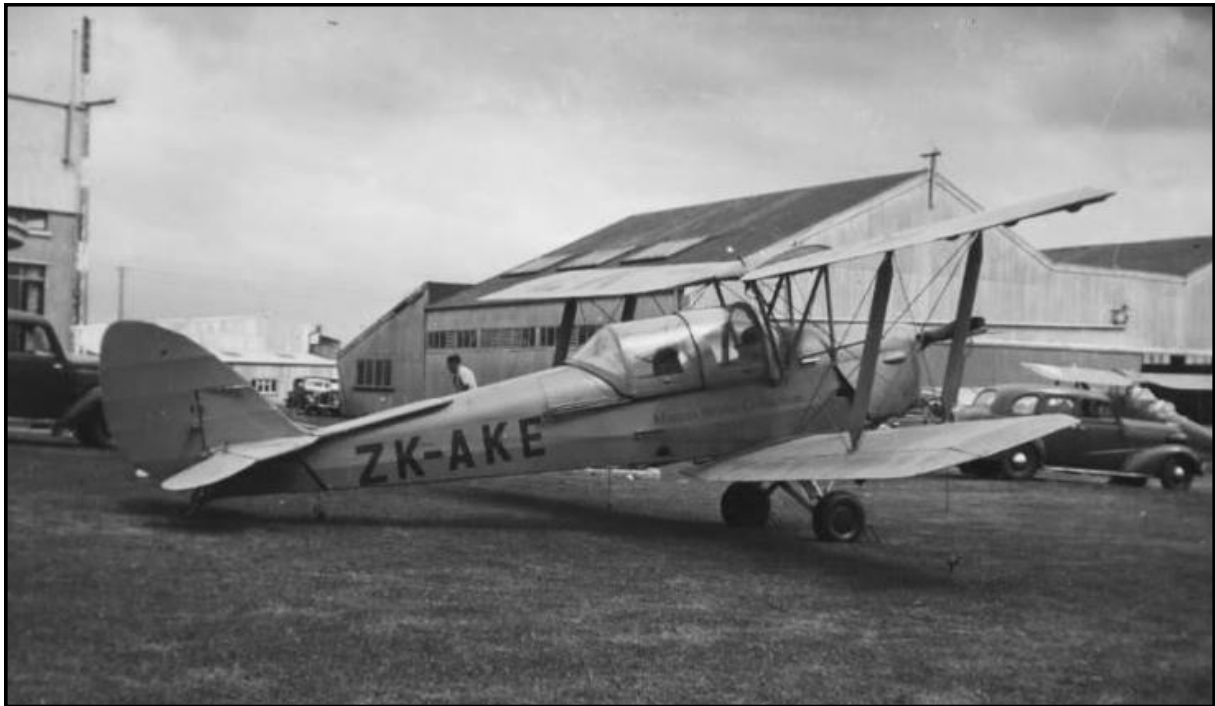
The first three cabin Tiger Moths in New Zealand had Canadian built canopies installed for the RNZAF
