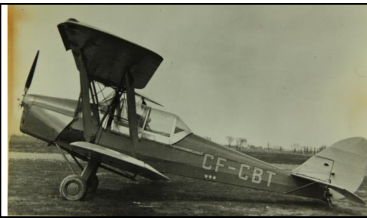
DH 82A built in UK & fitted with canopy in Canada
