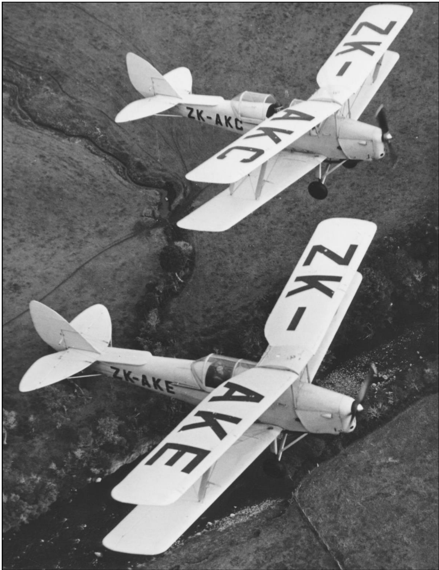
One of the biggest advantages of the Canadian-built canopies was that they could be flown either enclosed or open as demonstrated by these two New Plymouth Aero Club machines.
