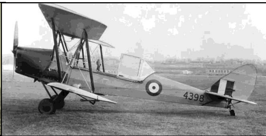
Canadian built DH 82C with canopy slid as far back as it would go Front sliding section goes over the top of the rear cockpit section Note the undercarriage stance, thinner interplane struts, tailwheel, and mass balance on aileron and elevator.
