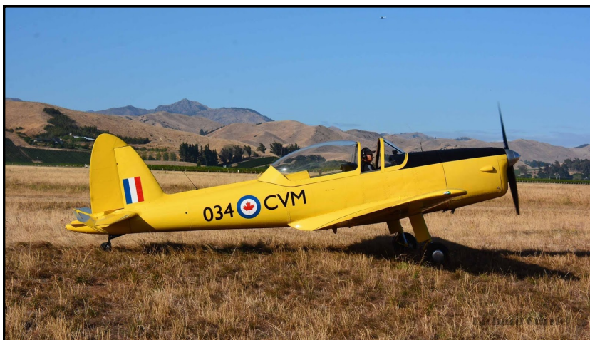
CVM fitted with a Canadian bubble type canopy.
