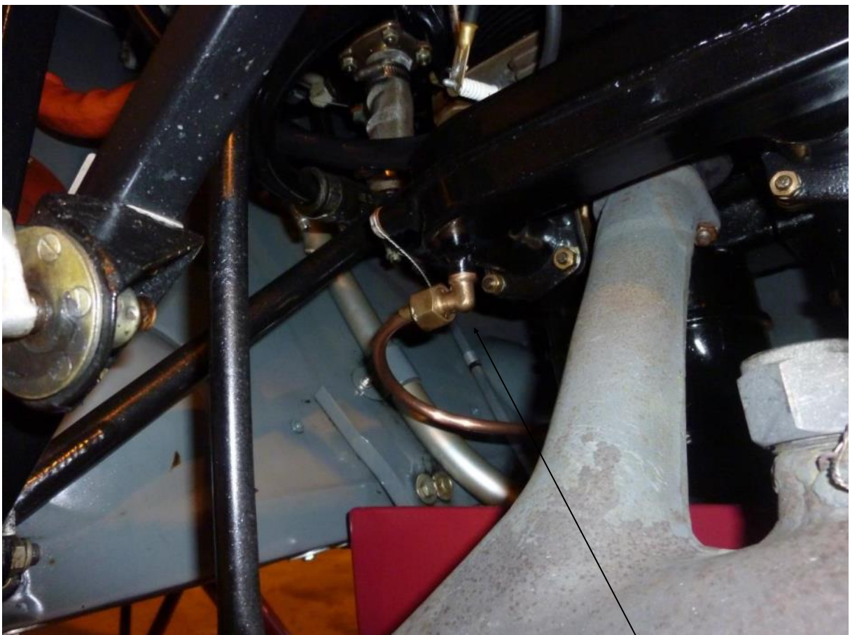
Manifold drain elbow
