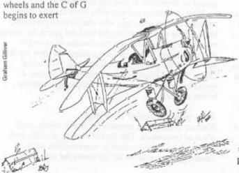
the sort of leverage that will easily win an argument with the elevator trying to hold it back. Friction between the grass and the wheels as they touch will tend to raise the tail anyway, and this effect will be greater touching down in a soft patch. Checking forward on the stick risks putting a Tiger on its back.
